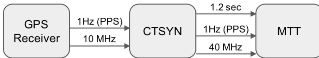
Figure 24.2: Central Timing synchronisation signals
