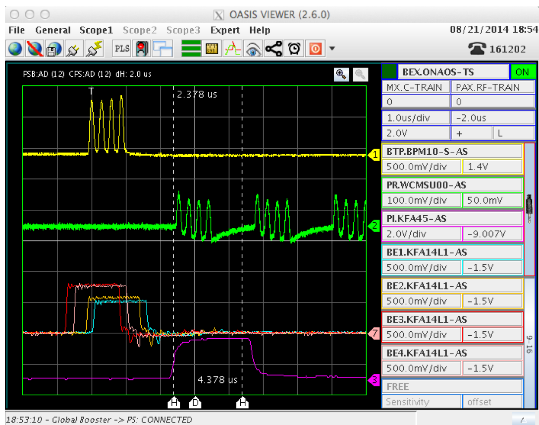
Figure 23.1: Virtual oscilloscope showing the transfer for PS Booster to PS
